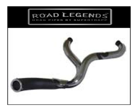
**CAUTION:** Due to the stylized features of this Paul Yaffe designed head pipe, there will be a loss of ground clearance during cornering, as compared to the stock system. Use caution when cornering with this system.
