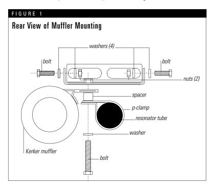
**7** Install P-clamp over resonator tube with flange facing U-shaped mounting bracket. It may be necessary to open the gap of the clamp with a channel lock, slide over the pipe, and then squeeze the flange ears together to re-align. Install 3/8"-16 X 2 bolt with 3/8" lock washer through P-clamp, spacer, muffler flange, and U-mount bracket. Snug bolt. Tighten remaining bolts in the following order:
