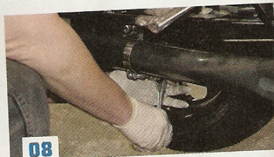
With the megaphone in place we tightened down the clamp that joined the muffer to the head pipes as per our instruction's specifications.
