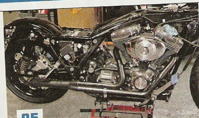
Here's a shot of the header pipes on the bike before the matching ceramic black megaphone and the heatshields went on.
