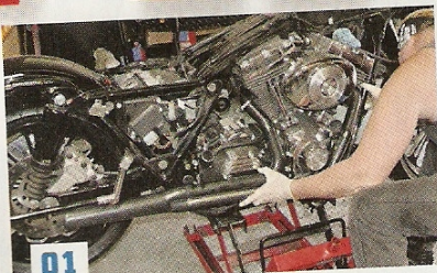
With the OE pipes removed, we slid the header pipes onto the front cylinder first, then the rear.
