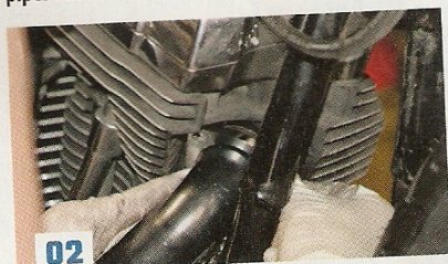
We snugged, but not tightened the head bolts on both the front and rear cylinders so we had a little wiggle room when installing the rest of the system.
