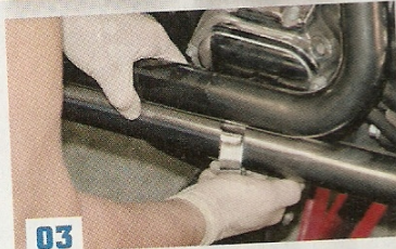
The pipes were attached to the OE pipe mounting bracket at the clutch actuation cover on the right side of the bike.
