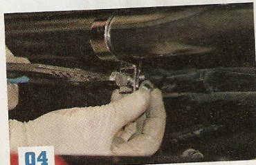
We then secured the clamp to the bike with the provided nut and bolt.
